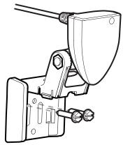
NOTE: Make sure that the mounting screws are snug, but do not fully tighten the mounting screws at this time to allow the transducer assembly to slide for adjustment purposes.
